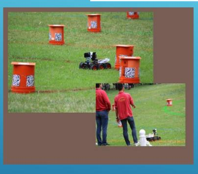
Each robot must be safely autonomous/
